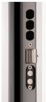
*The "motorised closing" system of every Matik model has a **door contact sensor**: an electronic device made of two contact points and installed in the fixed frame of the door, which lets the lock decide if the door is closed or open.*
